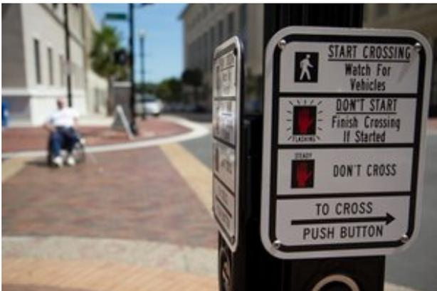
*Pictured:* Audible Pedestrian Signals provide non-visual directional information to pedestrians at intersection in Jacksonville, FL.
